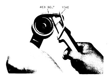
Fig. 4—Correct Positioning of 514-Type Tool
