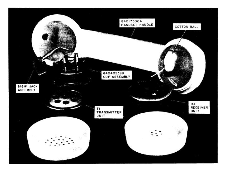
Fig. 3—G15A Handset Assembly (Current Version) or G15A Handset Assembly Converted from Current Version G3-Type Handset
