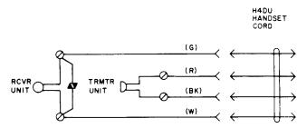
Fig. 8—\$G15Y Handset, Internal Connections\$
