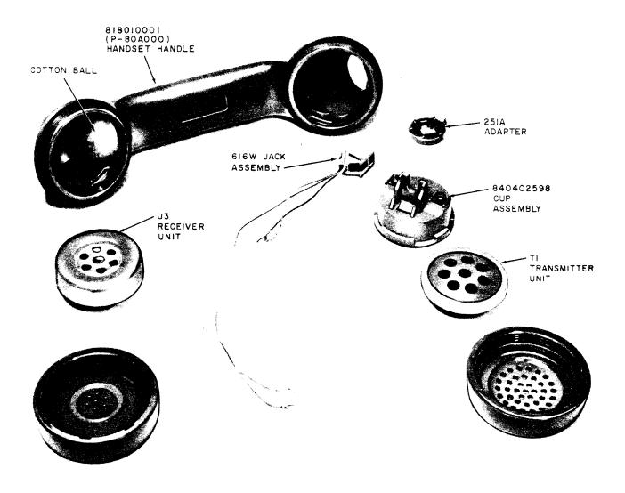
Fig. 4—G15A Handset Assembly Converted from Early Version G3-Type Handset
