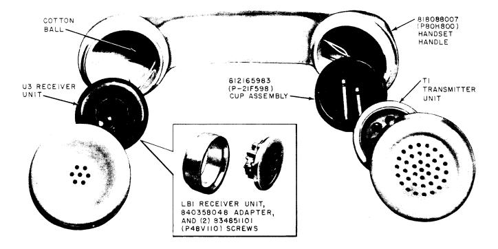
Fig. 2—G12A (A&M Only) Handset Assembly
