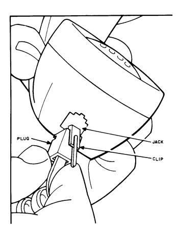
Fig. 6—Installing Handset Cord in G15A or G15Y Handset
