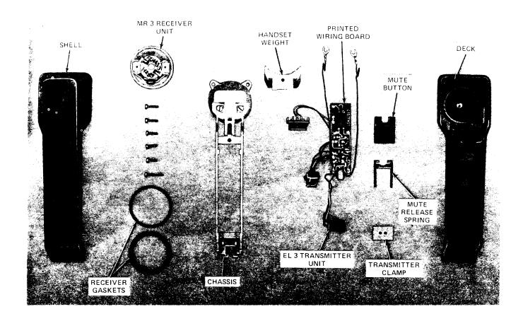
Fig. 6—R8C3 Handset, Interior View
