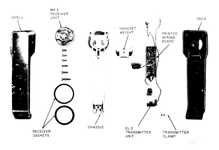
Fig. 5—R6C3 Handset, Interior View
