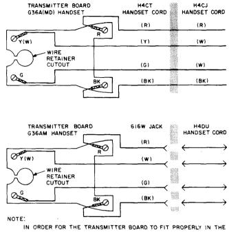
IN ORDER FOR THE TRANSMITTER BOARD TO FIT PROPERLY IN THE HANDSET, THE SPADE-TIPPED LEADS OF THE HANDSET CORD AND/OR JACK MUST BE PROPERLY POSITIONED ON THE BOARD AS SHOWN ABOVE.
