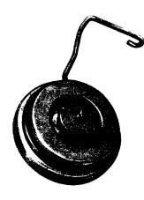
Fig. 25—664D Transmitter, Less Componenet Board
