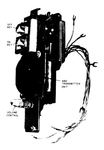
Fig. 27—667A (MD) and 667B Transmitter
