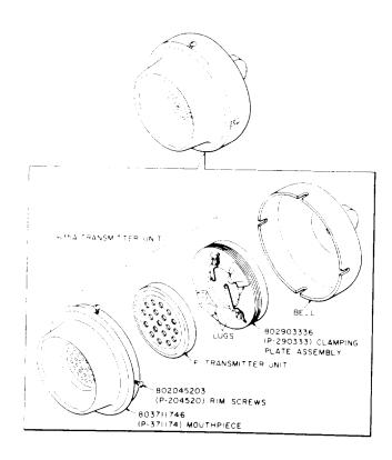
Fig. 14—635A Transmitter Unit
