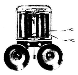
Fig. 3—B-Type Ringer Equipped With Gongs
