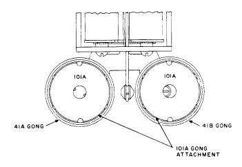
Fig. 4-101A Gong Attachment on B-Type Ringer
