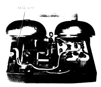
Fig. 5—Top View, Inside Wire Entering through Rear
