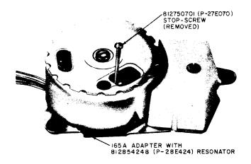
Fig. 3—P-Type Ringer Mounted on 165A Adapter
