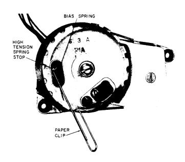
Fig. 6—Positioning Bias Spring
