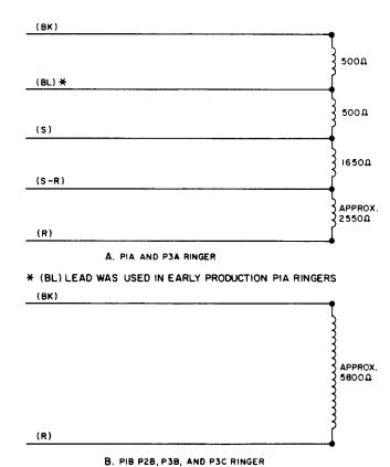
Fig. 5—▶P-Type Ringer—Schematic¶
