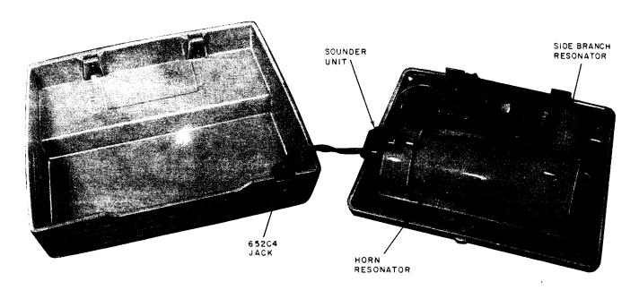
Fig. 3—♦S1AM Tone Ringer, Cover Removed♦
