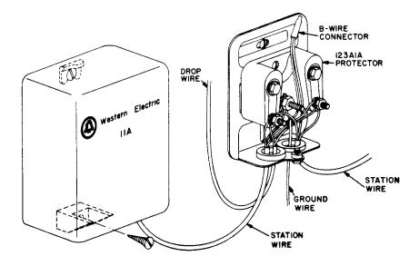
Fig. 1—11A/B Extender, Typical Installation
