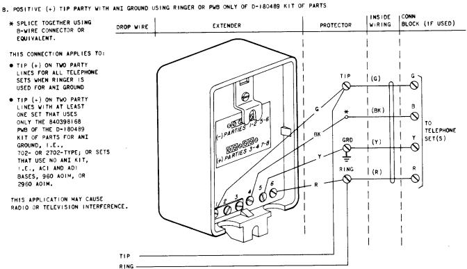
Fig. 4—11A/B Extender Connections for ANI Ground With Positive (+) Superimposed Ringing
