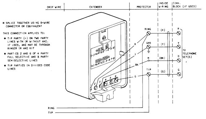
Fig. 2—11A/B Extender Connections with Negative (-) Superimposed Ringing
