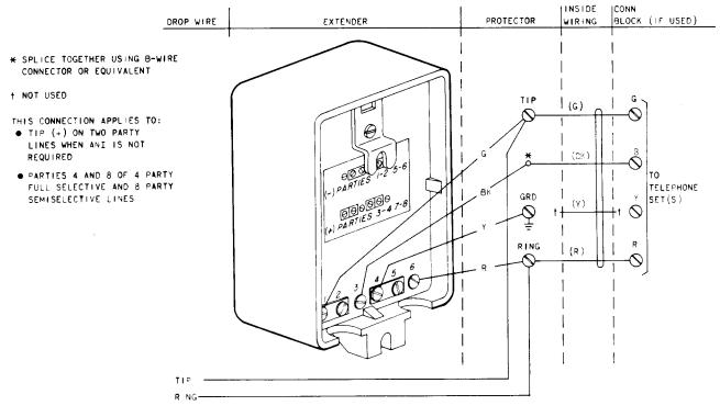
Fig. 3—11A/B Extenter Connections with Positive (+) Superimposed Ringing
