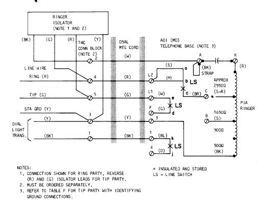
Fig. 6—Ringer Isolator Connections for AD1 (MD) Telephone Base With 220A (MD), 220AM, 2220B (MD) and 2220BM Hand Telephone Sets
