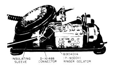
Fig. 2—Ringer Isolator in 500-Type Telephone
