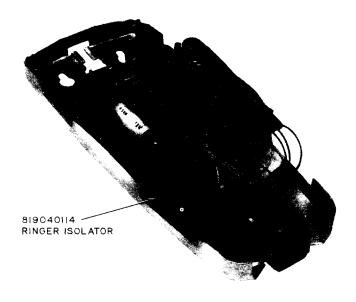
Fig. 4—Ringer Isolator in AC-Type Telephone Base
