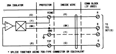
Fig. 3—28A Isolator Connections for Ring Parties (4-Conductor Wiring)
