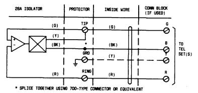
Fig. 4—28A Isolator Connections for Tip Party (4-Conductor Wiring)
