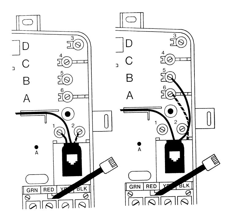
Fig. 2—Wiring the modular jack when installing the ANI-911 in an SNI-2100
