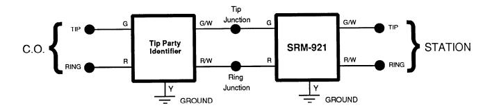
Fig. 2—Block diagram showing SRM-921 wired in conjunction with a Tip Party Identifier
