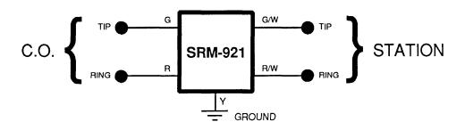
Fig. 1—SRM-921 Lead designations and connections
