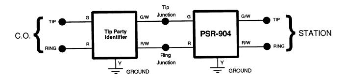
Fig. 2—Block diagram showing PSR-904 wired in conjunction with a Tip Party Identifier
