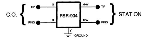
Fig. 1—PSR-904 Lead designations and connections
