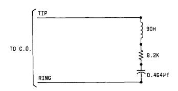
Fig. 2—▶1A Termination Unit, Connections •
