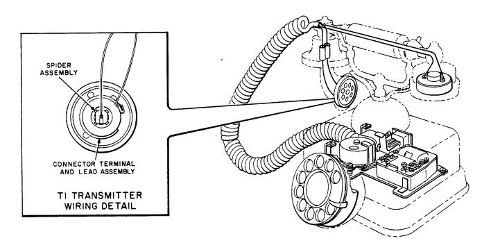
Fig. 3—Typical Installation of F-56659 or F-56660 Telephone Set in Antique Housing
