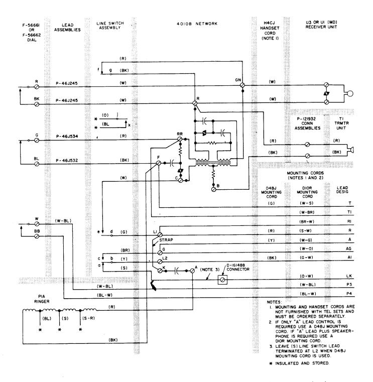
Fig. 5—F-56659 and F-56660 Telephone Set, Wired For 1A1 or 1A2 KTS and 3-Type Speakerphone
