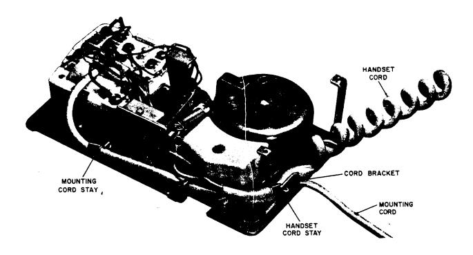
Fig. 2—Installation of Mounting and Handset Cords
