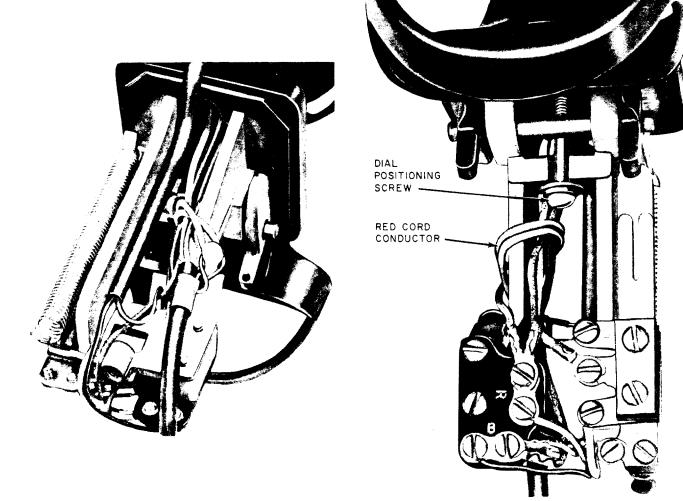
Fig. 9—Wiring of Hangup-Type Hand Telephone Set
