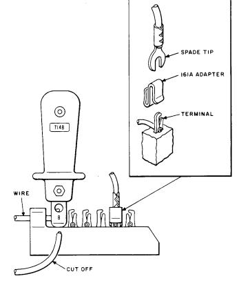
Fig. 16—Terminating Station Wire and Spade Tip
