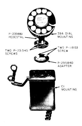
Fig. 8-39A Dial Mounting With C1 Handset Mounting
