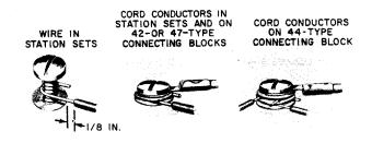
Fig. 15—Terminating Station Wire and Cord Conductors on Screw Type Terminal
