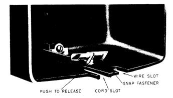
Fig. 11—Entrance Hole in Housing of 554 Wall-Type
