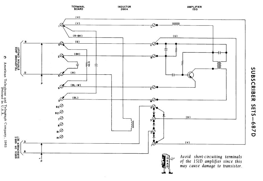
Fig. 1 - Circuit Diagram for Connection with Telephone Jack Station
