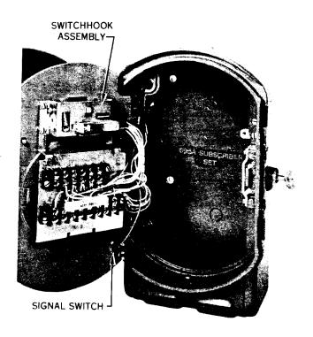
Fig. 3 — 695A Subscriber Set, Outer and Inner Door Open
