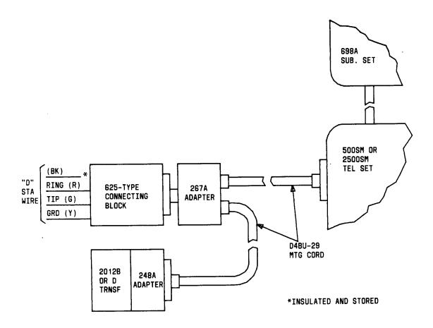
Fig. 6—Code-Com Set Without KS-20614 Relay Switch
