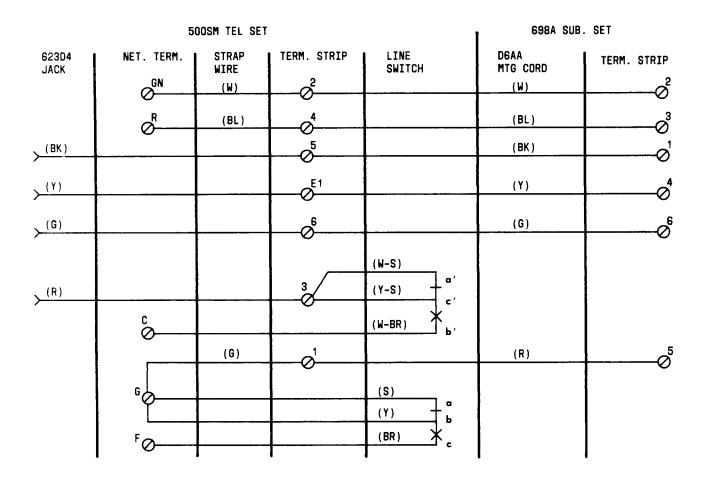
WIRING MODIFICATIONS, 500SM TEL SET TO PROVIDE DIRECT CONNECTIONS TO 698A SUB. SET
