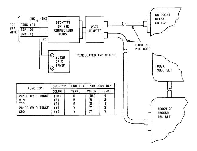
Fig. 5—Code-Com Set With KS-20614 Relay Switch
