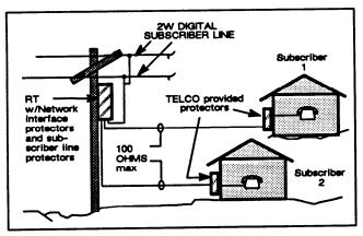
Figure 1. Typical DDL112 Installation
