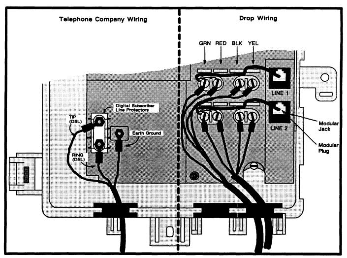
Figure 4. Partial Drawing of Remote Terminal Enclosure Showing Wiring
