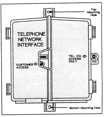
Figure 2. DDL112 DuaLine Plus Remote Terminal in the Secured Position (Closed)
