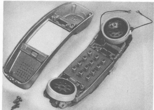
Fig. 13—Field Coil Installed in Receiver Cup of Chassis Assembly
