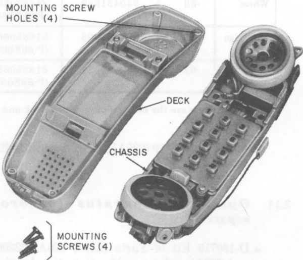
Fig. 7—2220C Hand Telephone Set With Chassis Assembly Removed from Deck
