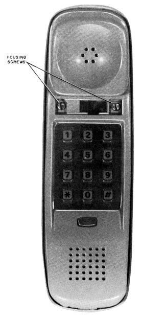
Fig. 6—Location of Housing Screws
