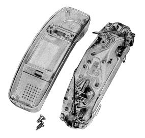
Fig. 17—Terminating Field Coil Leads to Receiver Cup Mounting Screws
