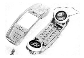
Fig. 14—Field Coil Installed in Receiver Cup of Chassis Assembly
