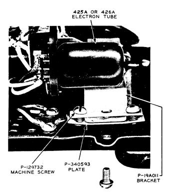
Fig. 7 — Electron Tube Bracket
