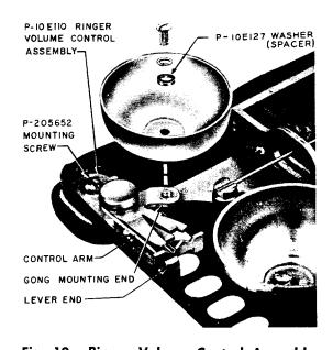
Fig. 10 - Ringer Volume Control Assembly
