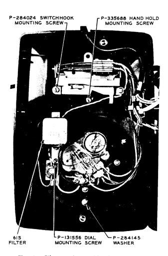
Fig. 8 — Filter and Switchhook Assembly
