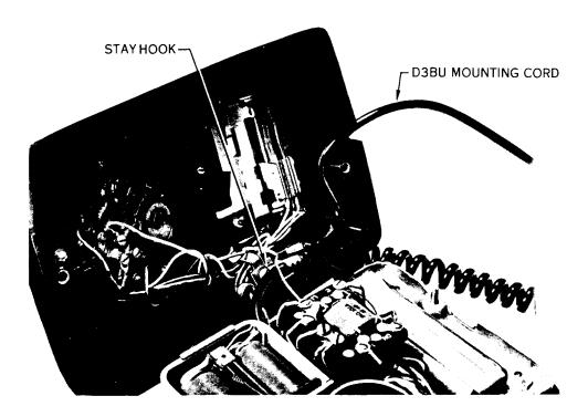
Fig. 5 — Installing D3BU Mounting Cord
