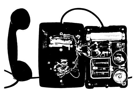
Fig. 2 - 5300 Series Telephone Sets, Interior View
