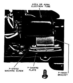
Fig. 1 - Electron Tube and Bracket
