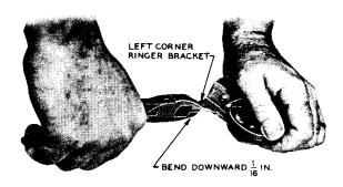
Fig. 4 — Method of Bending Left Ear of Ringer Bracket
