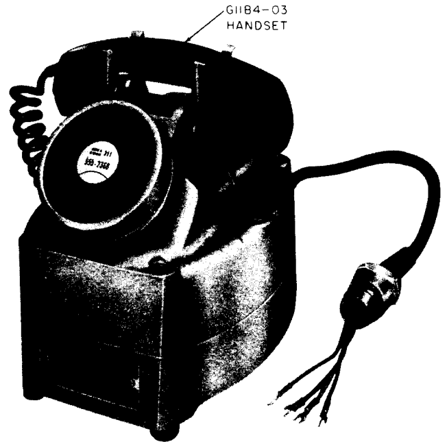
Fig. 1—KS-14476, List 2 Manual Telephone Set
