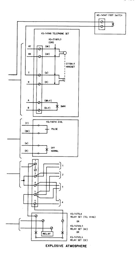
Fig. 8—KS-14548 Telephone Set, Connections (Sheet 2 of 2)
