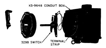
Fig. 4—KS-14547 Foot Switch, Interval View
