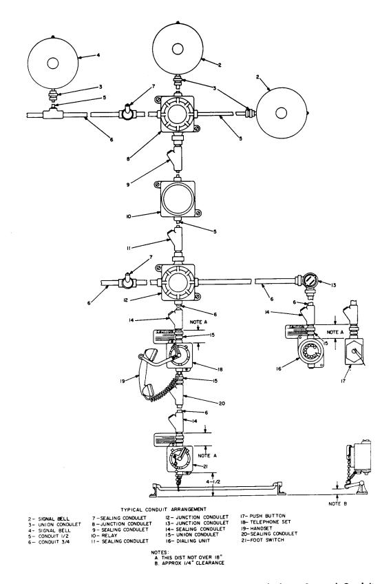
Fig. 2—Typical Arrangement Involving the KS-14548 Telephone Set and Conduit
