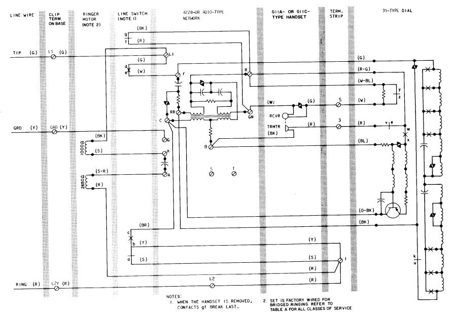
Fig. 5—2520B Telephone Set, Connections
