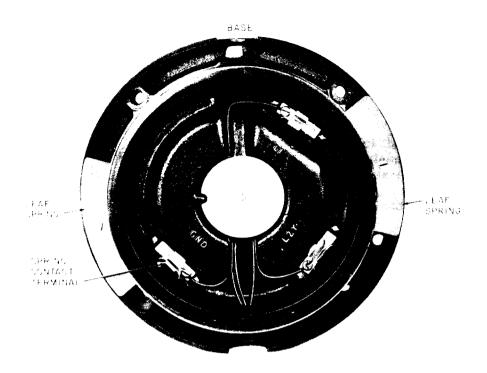
Fig. 3—Local Wiring in Base
