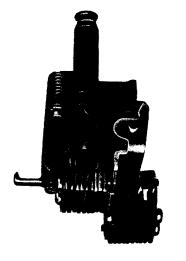
Fig. 3 – Exclusion Key Assembly Removed from Set (Key in Operated Position)
