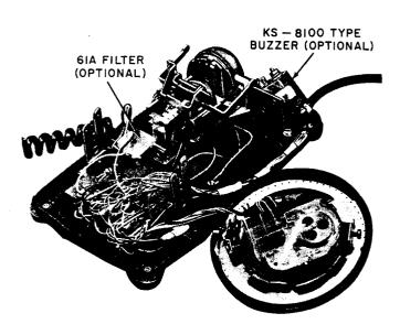
Fig. 2—529B Telephone Set, Interior View
