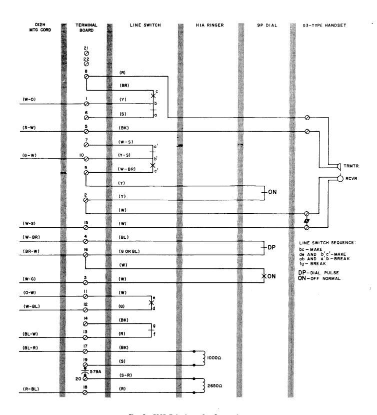
Fig. 3—529B Telephone Set Connections
