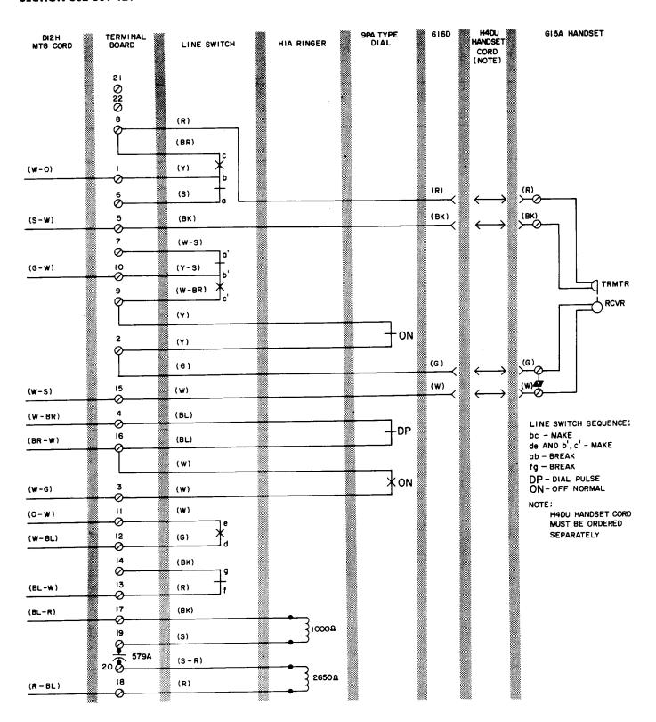
Fig. 4—♦529BM Telephone Set Connections ♦
