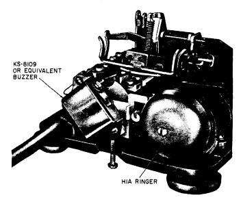
Fig. 9—Location of KS-8109 Type Buzzer
