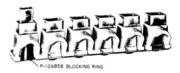
Fig. 8—P-12A858 Blocking Ring Installed
