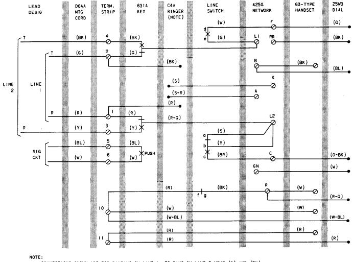
CONNECTIONS SHOWN ARE FOR RINGING ON LINE 1. TO RING ON LINE 2, MOVE (R) AND (BK) RINGER LEADS TO TERMINALS 3 AND 4. TO SILENCE RINGER, CONNECT (BK) TO K TERMINAL. LINE SWITCH SEQUENCE: bc - MAKE de - MAKE
