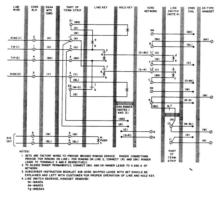
Fig. 1—1515B (MD) Telephone Set, Connections With 25W3 (MD) Dial4
