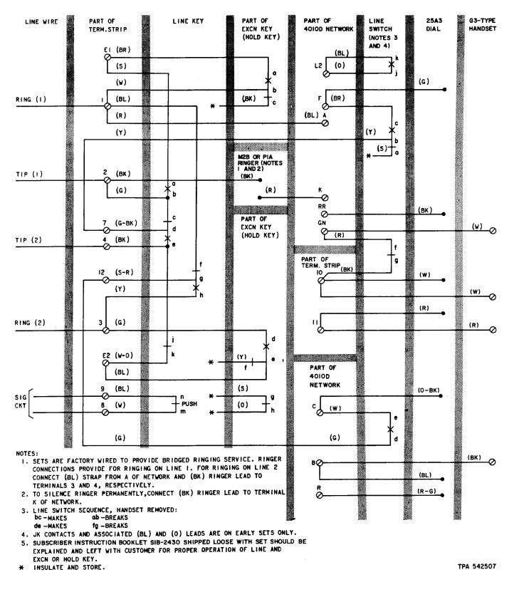
♦Fig. 2—1555B Telephone Set, Connections With 25A3 (MD) Dial∉
