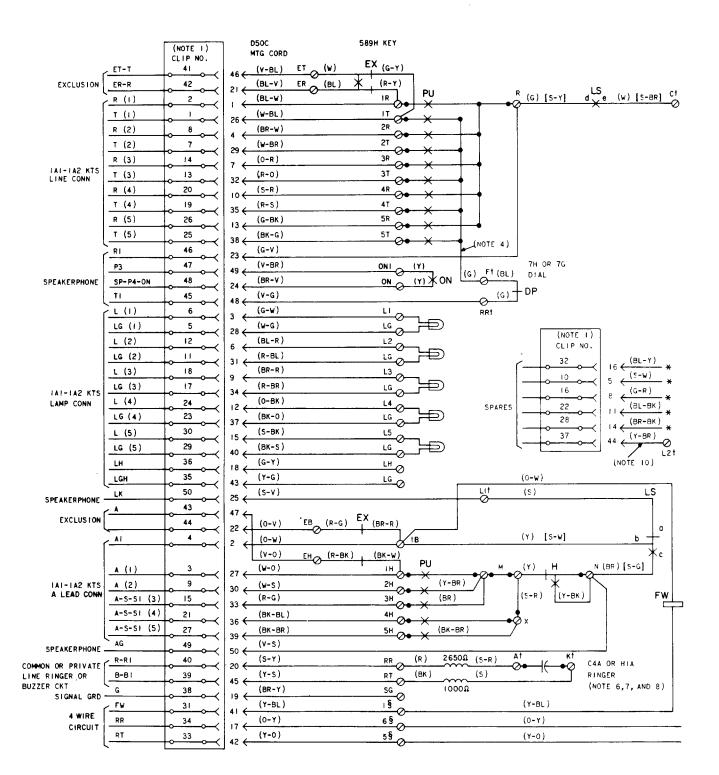
Fig. 1—568HB Telephone Set, Connections (Sheet 1 of 2)
