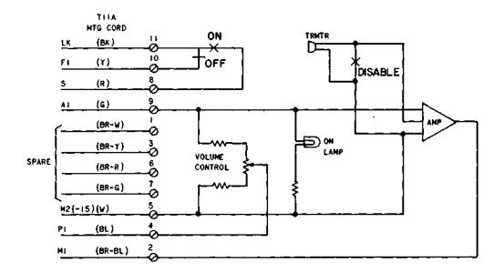
Fig. 3-666A (MD) Transmitter Connections
