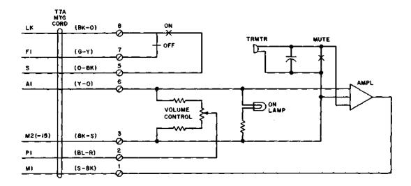
Fig. 4-666B Transmitter Connections
