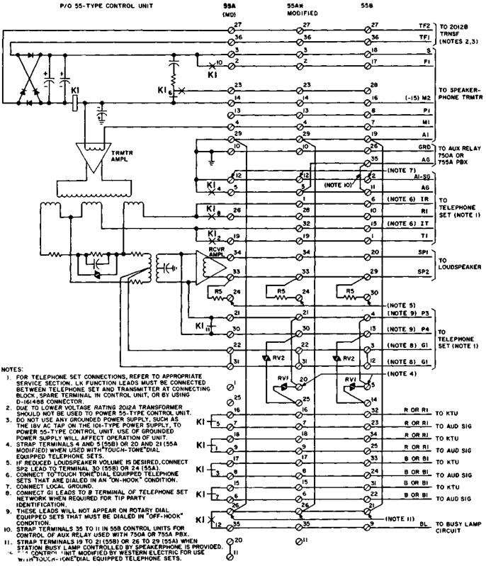
Fig. 2—55-Type Control Unit Connections
