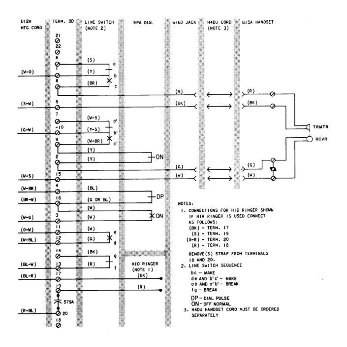
Fig. 2—♦529BM Telephone Set, Connections
