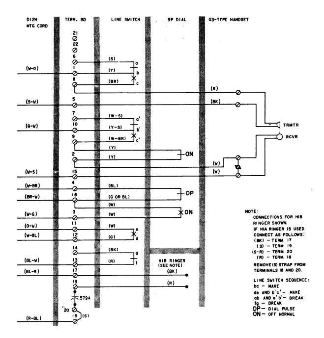
Fig. 1—♦529B Telephone Set, Connections¢
