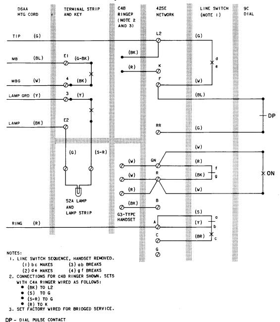
Fig. 1-516B Telephone Sets, Connections
