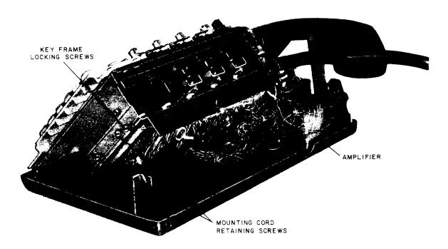
Fig. 26—Key Frame Raised on Early Production Telephone Set
