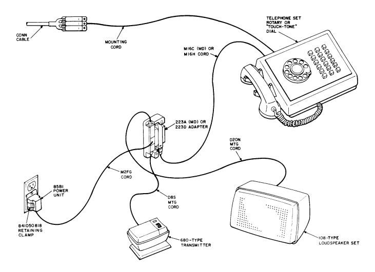
Fig. 20—♦4A Speakerphone System Arrangement, CALL DIRECTOR Telephone Sets Using 223A (MD) or 223D Adapter
