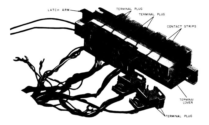
Fig. 8-Typical Connections to 635-Type Key
