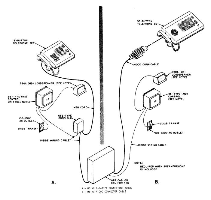
Fig. 21—Two Typical Installation Layouts (Including Speakerphone)
