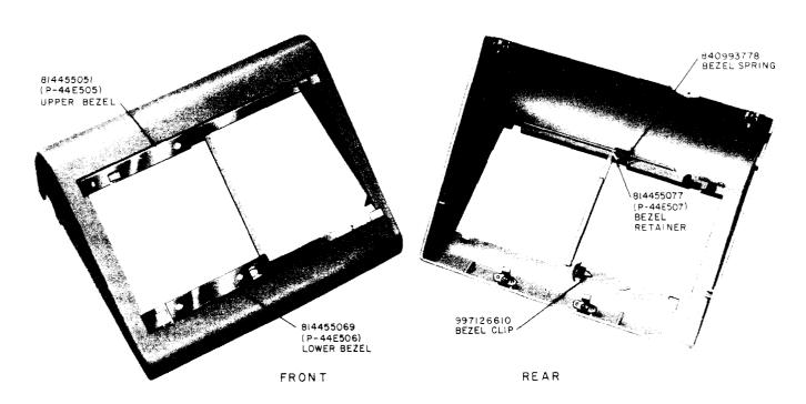
Fig. 4—Housing With Two-Piece Bezel Assembly Installed
