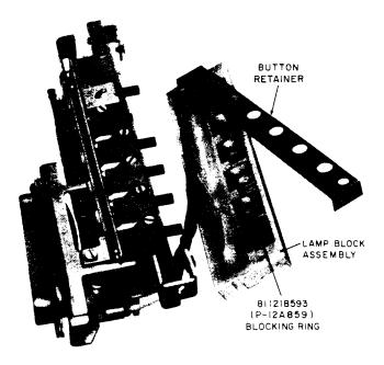
Fig. 12—Blocking Ring Installed in 590 or 650 Series Keys
