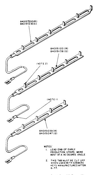
Fig. 9—Contact Strip Used With 635-Type Keys
