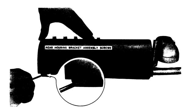
Fig. 6—Housing Retaining Screws
