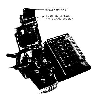
Fig. 18—Mounting Location For Second KS-8109L2
