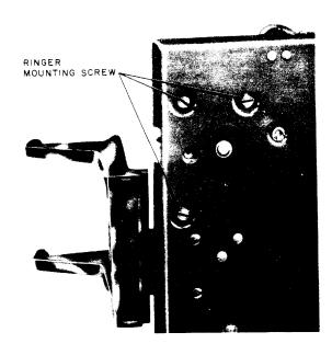
Fig. 27—Location of Mounting Screws for N1A or T1A Ringers
