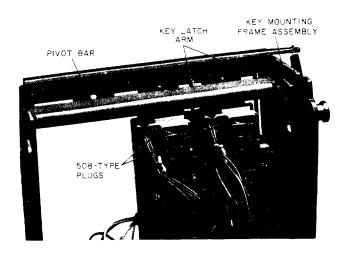
Fig. 29—Rear View of Pivot Bar (Current Production Set Equipped With 635-Type Keys)
