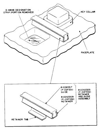
Fig. 24—812263325 (P-22F332) Retainer and Guide Assembly—Enlarged Cutaway End View
