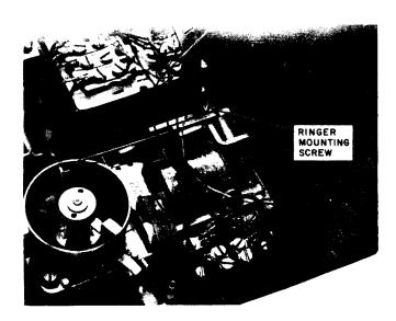
Fig. 28—Location of Mounting Screws for D1-Type
