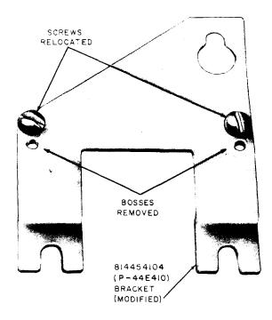
Fig. 17—Buzzer Mounting Bracket Assemblies
