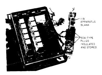
Fig. 14—Insulating and Storing 508-Type Plugs on 111B Apparatus Blank
