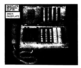
Fig. 3—₱Installing 2621A Faceplate on 30-Button CALL DIRECTOR Telephone Set ■
