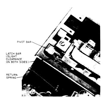
Fig. 7—Positioning 590 and 650 Series Keys
