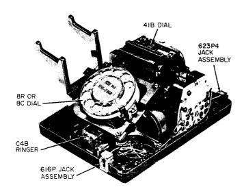
Fig. 2-660A1M Telephone Set Base
