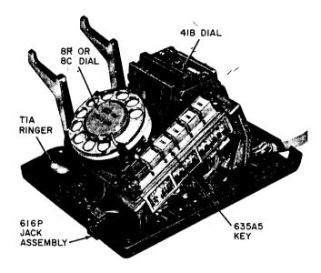
Fig. 2—662A1M, Telephone Set Base
