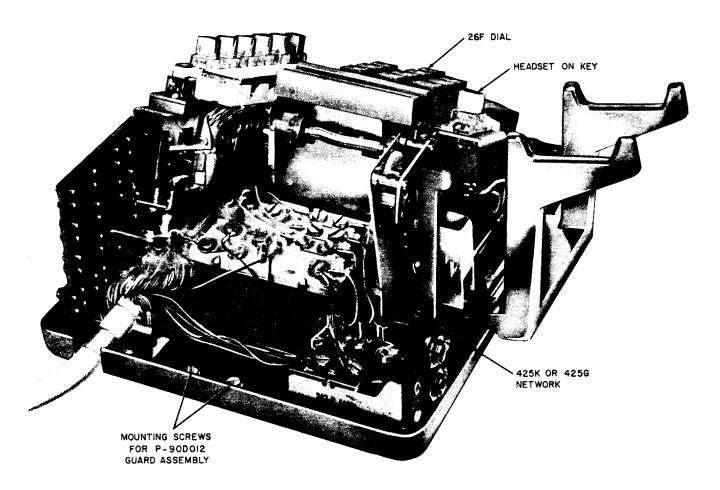
Fig. 5—1664B1 Telephone Set, Housing Removed
