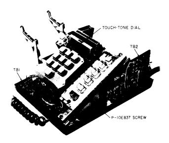
Fig. 4—1662-Type Telephone Set, Housing Removed
