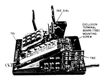
Fig. 3—2662A1 Telephone Set, Housing Removed
