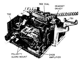
Fig. 4—2664A1 Telephone Set, Housing Removed
