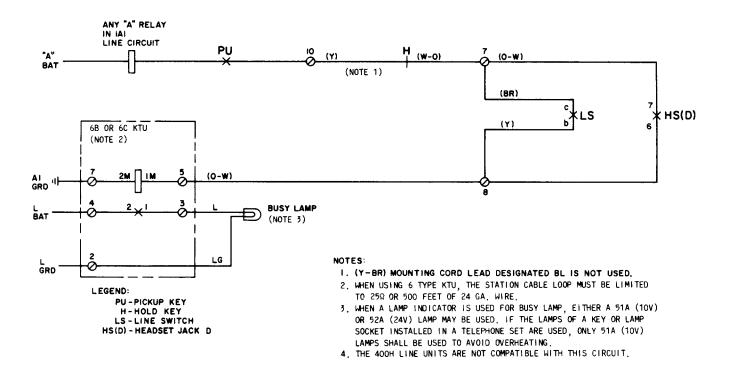
Fig. 6—Busy Lamp Control Circuit Associated With 1A1 and 1A2 KTS (Note 4)
