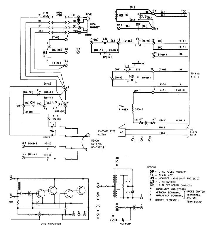
Fig. 2—636CAMS and 637DAMS Telephone Set, Connections
