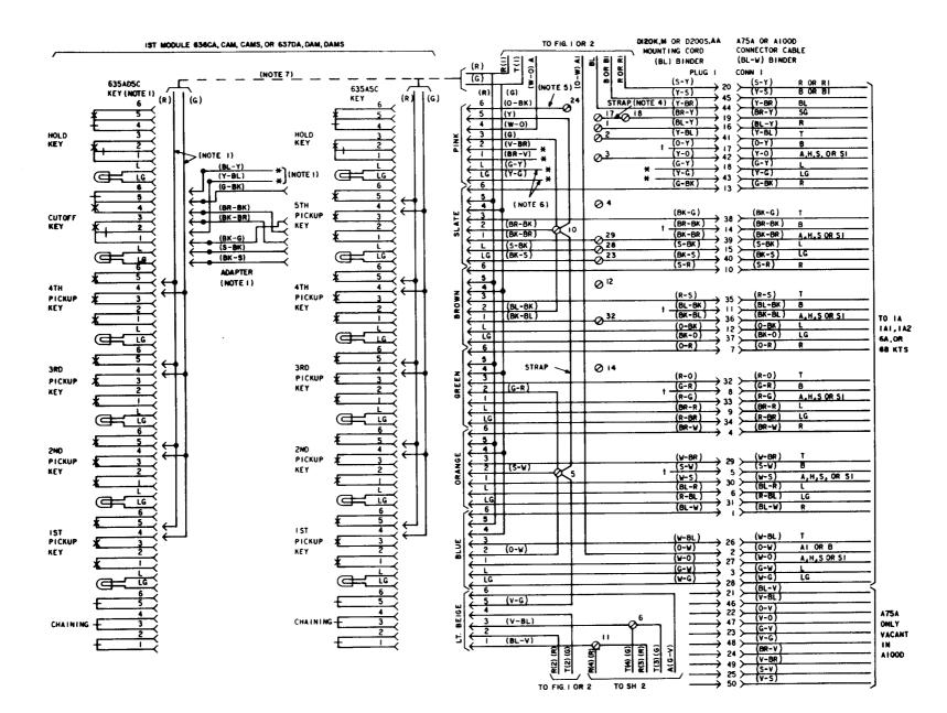
Fig. 3-Module and Connector Cable Arrangements (Sheet 1 of 5)
