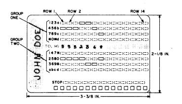
Fig. 3—Dial Card Coded For 7-Digit Telephone Number
