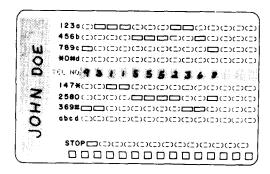
Fig. 4—Dial Card Coded for Access Code (9), Stop, Area Code (311), and 7-Digit Telephone Number
