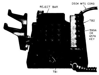
Fig. 2—F-58555 Telephone Set, Interior View
