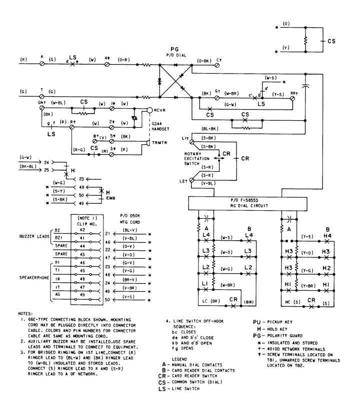
Fig. 5—F-58555 Telephone Set Connections (Sheet 2 of 2)
