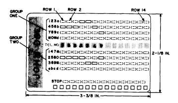
Fig. 3—Dial Card Coded for 7-Digit Telephone
