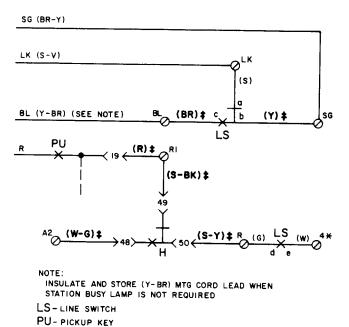
Fig. 6—1A KTS and Station Busy Lamp Modifications
