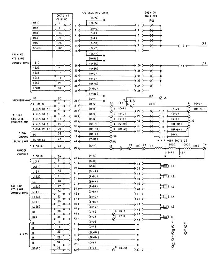
Fig. 5—F-58555 Telephone Set Connections (Sheet 1 of 2)
