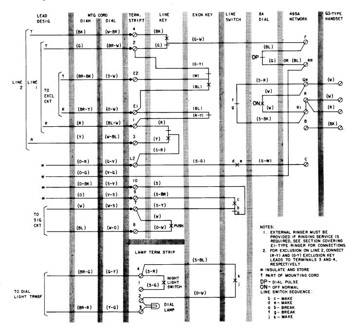
♦Fig. 1—711B (MD) Telephone Set Connections wired for 2-Line Pickup, Exclusion on Line 1¢
