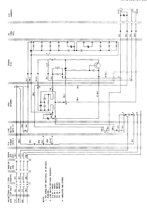
Fig. 11—2910A Telephone Set, Connections
