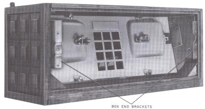
Fig. 9-\$2910A Telephone Set with Telephone Set Base Removed
