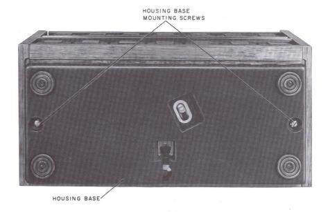
Fig. 7—Removing Metal Housing Base (910A or 2910A Telephone Set)
