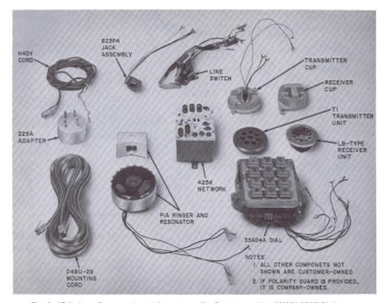
Fig. 6—Telephone Company-Owned Components (Set Equipment with a TOUCH-TONE Dial)
