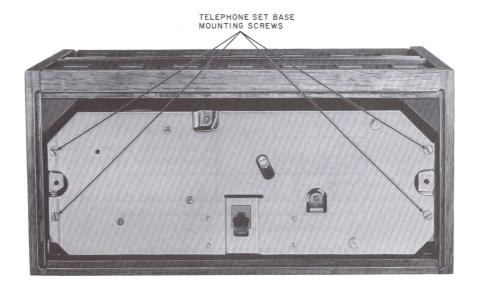
Fig. 8—Removing Telephone Set Base (910A or 2910A Telephone Set)
